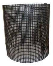
Step 3 Attach the mesh cylinder to the inside circumference of the hole in the center of the float. There are 1/4-20 brass inserts molded into the float to attach the debris screen. Secure the debris screen with stainless steel  $1/4-20 \times 1/2$  inch hex head screw and a 1/4 inch stainless steel washer.
